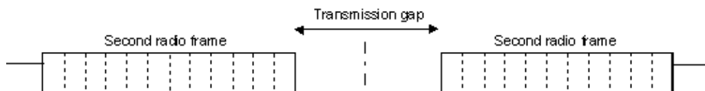
Fig. 5-8: Envelope of compressed mode signal with double-frame method
